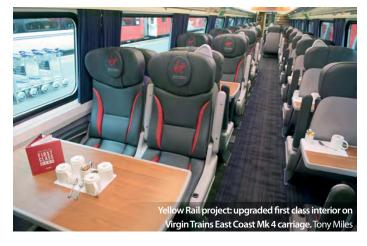
and table pedestals, fitment of new body side and dado panels, provision of replacement seat cushions and covers, on-board signage, new saloon and vestibule carpets, replacement lino, tables and renovation of the toilets. In addition, first class carriages benefit from the fitment of leather seats and mood lighting.
