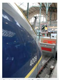
Stopping aid: mirror to guide Class 374 trains to stop in the correct place in Paris Nord. Keith Fender
